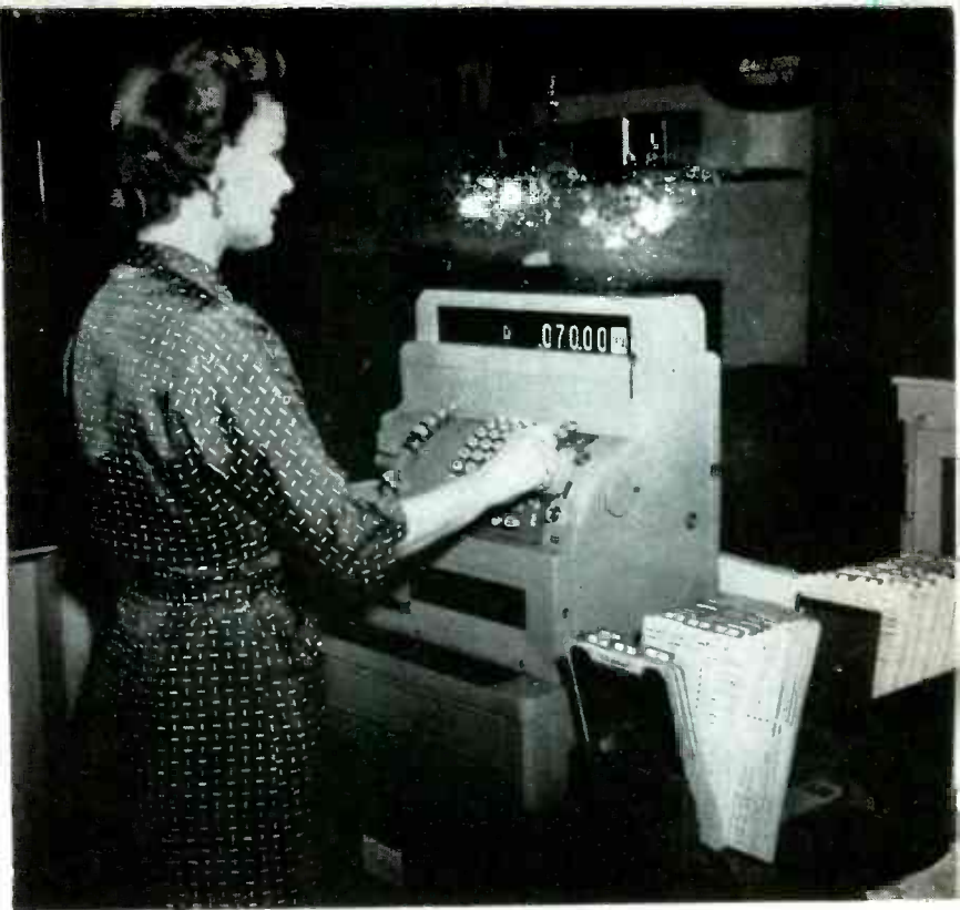
(Above) The bookkeeper posts a transaction. The machine accumulates totals of nine types of transactions.
