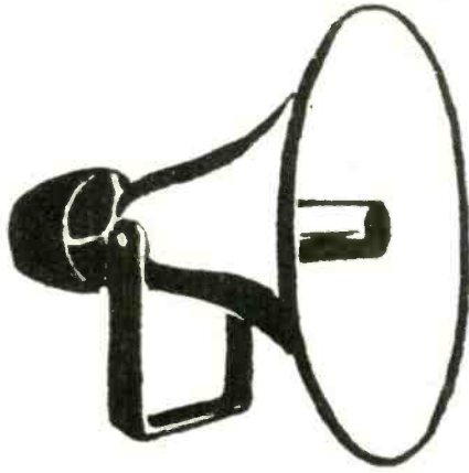
Fig. 4—Typical reentrant trumpet with 20" bell diameter.
