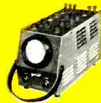
Philco 3" oscilloscope—Model S-8200. Portable or for use on the bench.
