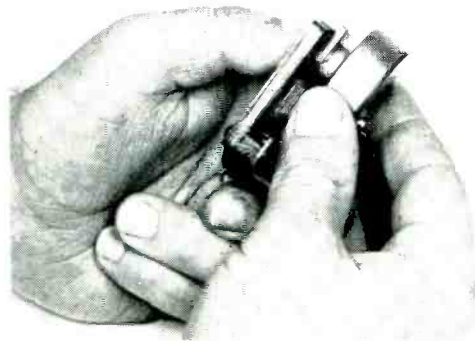
Fig. 2—You need only to take out two screws in order to remove the rotor.
