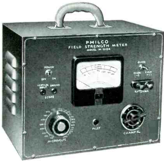
Field Strength Meter
