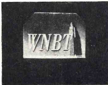
Fig. 7. Vertical foldover resulting from faulty condenser.
