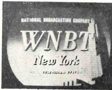
Fig. 4. Blurred picture caused by leaky video amplifier condenser.
