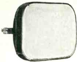
16RP4 original studio-matched rectangular picture tube.
