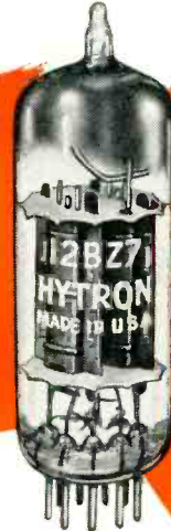
← NEW 12BZ7 High-mu, 9-pin miniature dual triode. Especially de- signed for sync. separators and sync. amplifiers, high- gain audio amplifiers, and gating circuits.
