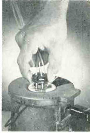
Fig. 3. Prongs and leads are immersed in pot.
