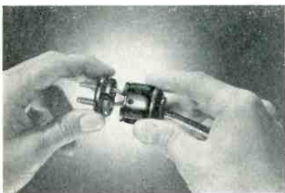
Fig. 5. Cap is slipped over wires and pushed over plug.
