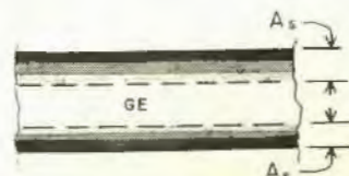
Fig. 2—Arsenic vapor diffusion through the germanium.
