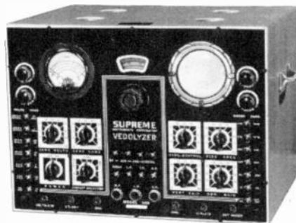
A "Vedolyzer" which uses a meter and oscillograph as indicators.
