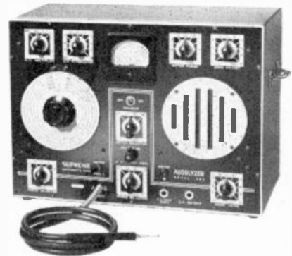
An "Audolyzer" which uses a meter and speaker as indicators.
