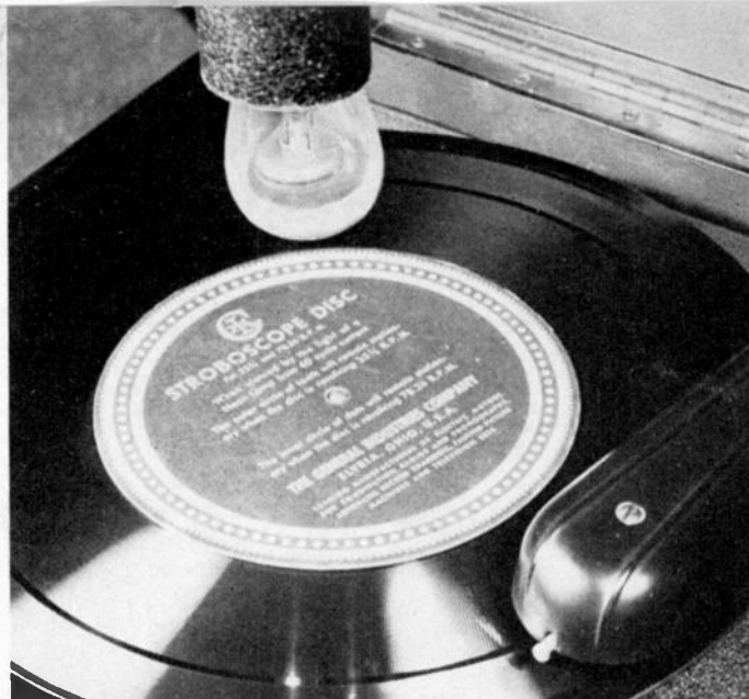
Set-up for checking speed of phonograph turntable with neon tube and stroboscope disc. Pickup is run through outside of record to establish normal load.
