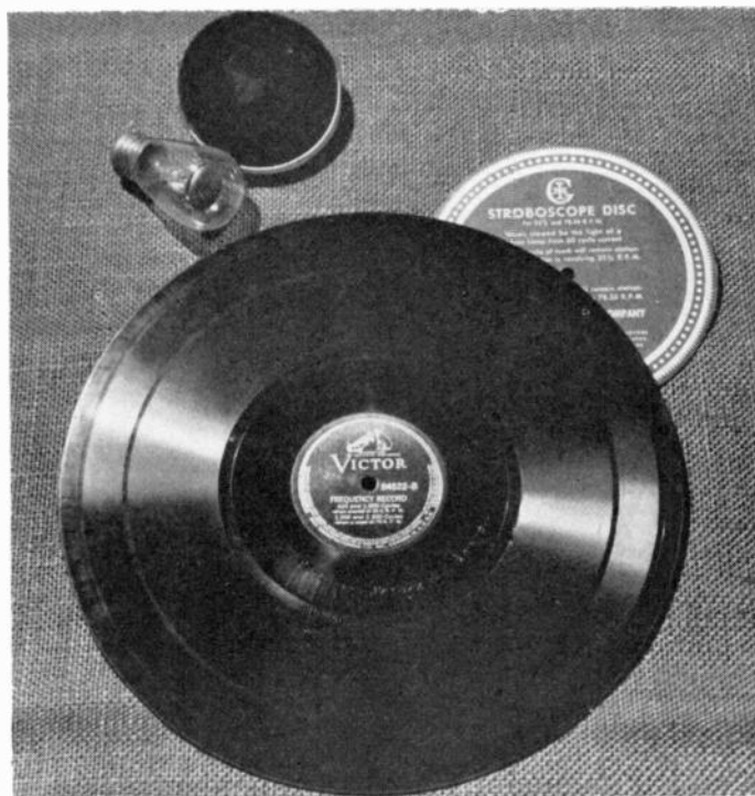
Equipment every serviceman should have—a frequency test record, a stroboscope disc, a neon tube for use with the disc, and a record cleaning pad. They're all handy and provide impressive tests.
