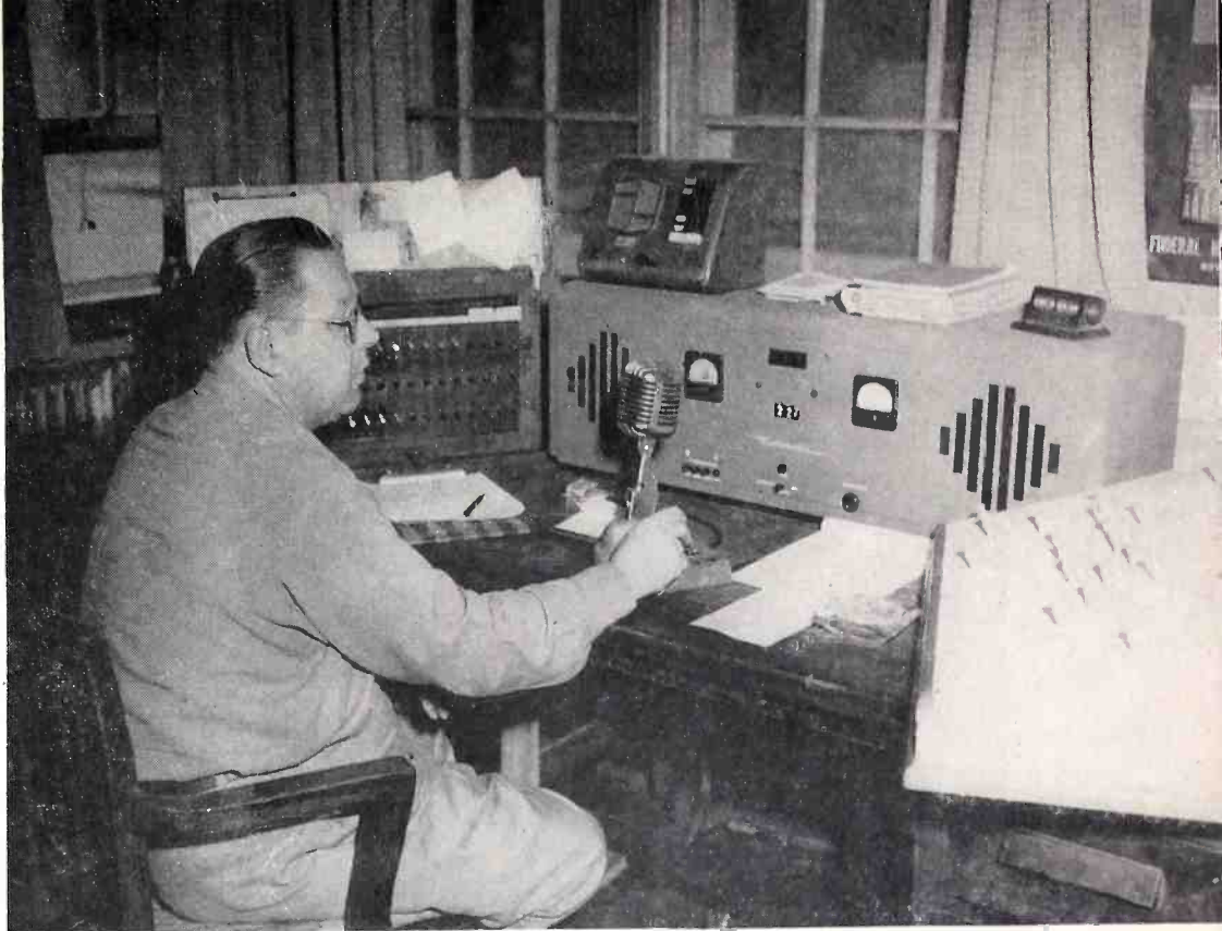
Fig. 1—A Motorola remote control unit operates the 50 watt FM transmitter of Madison's Yellow Cab Co. The transmitter is located two miles away on top of one of Madison's highest buildings. The dispatcher is Harold Hussy.
