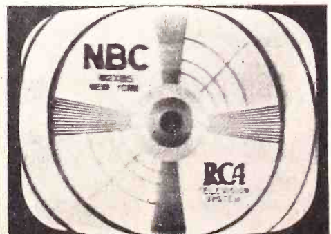
Fig. 2b—Pattern with H.F. distortion.
