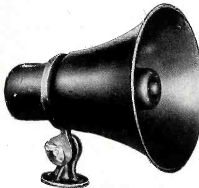
NEW SMALL RE-ENTRANT HORNS , extremely efficient for factory inter-com and paging systems; for sound trucks, R.R. yards and all other industrial installations where high noise levels are prevalent. Watertight, corrosion-proof, easily installed. Two new models — type RE-1 1/2, complete with Baby Unit, handles 25 watts, covers 300-6000 cps; type RE-12, complete with Dwarf Unit, handles 10 watts, freq. response of 400-8000 cps.
