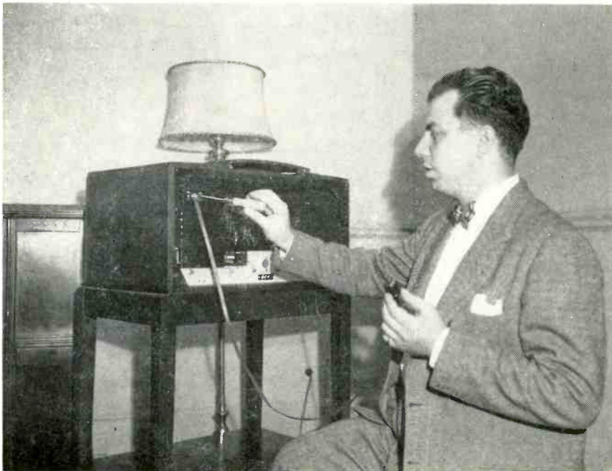
Fig. 5—The author demonstrates how simple it is to connect the TV receiver to line that connects to outlet.
