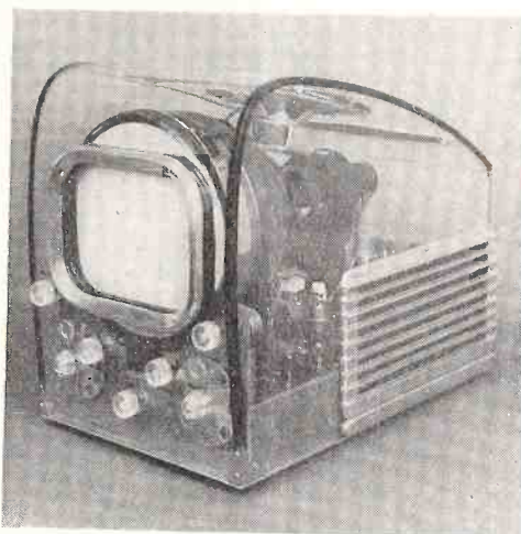
Above: Phantom view, Farnsworth FV-200 table telereceiver; cased model below, in metal cabinet. (See text).
