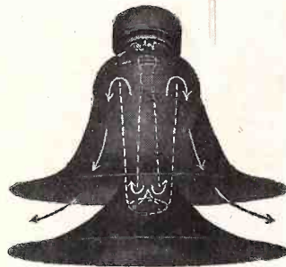
RADIAL HORN SPEAKER; a 3\frac{1}{2} " re-entrant type horn. Projects sound over 360^\circ area. Storm-proof. Made of RACON Acoustic Material to prevent resonant effects.
