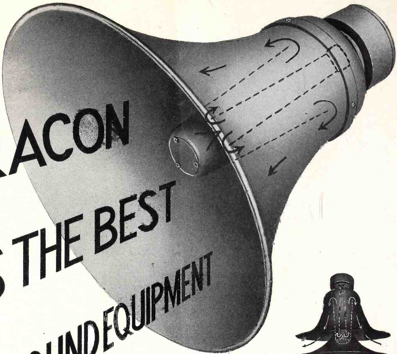
RADIAL HORN SPEAKER; a 3½' re-entrant type horn. Projects sound over 360° area. Storm-proof. Made of RACON Acoustic Material to prevent resonant effects.
