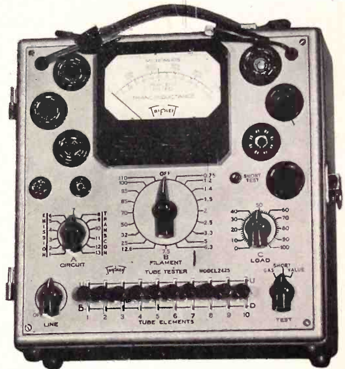
Figure 3 (right). Triplet 2425 principle: "Grid bias is directly proportional to the grid to plate transconductance . . ." (See text).
