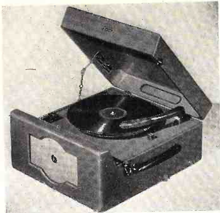
Emerson Portable Phono Model 521. Three tube amplifier, increased power output with new circuit; 6½-inch Alnico 5 PM dynamic speaker; crystal pickup; self-starting constant speed motor. Plays all sizes records with lid closed.
