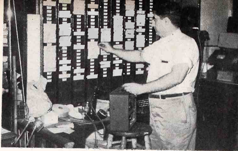
Time-card rack is used for job tickets and tags. Job number tag is taken off the radio receiver when work is completed.
