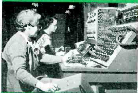
This operation gives a percentage of all previously tested tubes a thorough going-over—just as a "double-check."
