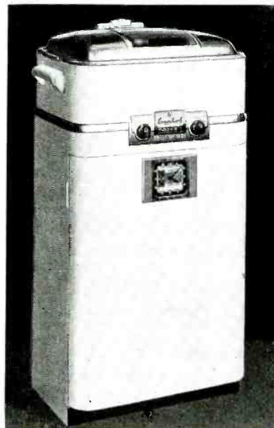
SWARTZBAUGH , Everhot model 900 roaster. Has Lock-In lid, moisture control, temperature guide, timer clock and cover lifter. Capacity 18 liquid and 20 dry pounds. White baked enamel finish. Operates on 115 volts A.C., draws 1320 watts. 40" high with cover closed. Cooking well 16" long, 11" wide and 5 1/2" deep. Swartzbaugh Mfg. Co., Toledo 6, Ohio.
