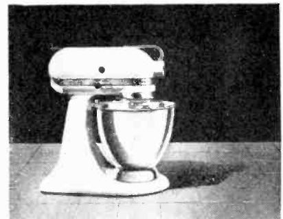
KITCHENAID , Top: Model K4-B food mixer; 10 definite (and intermediate) speeds, governor-controlled. Universal type 1/6 h.p. motor, operates direct through steel cut gears. Variable speed attachment hub on front of mixer for accessories. Standard equipment: one 4-qt. finned steel mixing bowl; wire loop whip; combination beater-pastry knife. Ht. 14"; base 8"x14"; weight 24 lbs. Below: Model 3-B; 1/4 h.p. motor; other specifications same as above. Standard equipment: one 3-qt. heat-resisting glass mixing bowl; juice extractor; all-purpose stainless steel beater for mixing, beating, whipping and making pastry. Other attachment priced separately. Ht. 13 3/4"; base 7 1/2"x12 3/8". Weight 18 lbs. Hobart Mfg. Co., Kitchen-Aid Div., Troy, Ohio.
