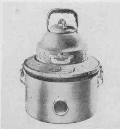
FILTER QUEEN Bagless vacuum cleaner; consists of a dust-pan, filter cone and power unit. 2/3 h.p. Black & Decker motor moves 40 cu. ft. of air per minute. Cellulose filter removes dust and dirt, drops into sealed, metal dust-pan. Comes with dust-brush, nozzle, crevice tool, shampoo and wax sprayer, demother. Health-Mor, Inc., Chicago, Ill.
