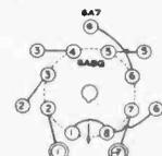
TYPE 6A7 REPLACING TYPE 6A8G
