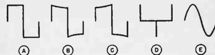
Figure 4. Various square-wave forms. "A" is perfect square-wave. "B" and "C" show low-frequency phase shift; "B" is poor low-frequency response, and "C" is high response at low-frequency. "D" shows extreme low-frequency attenuation, while "E" pictures a high frequency attenuation
