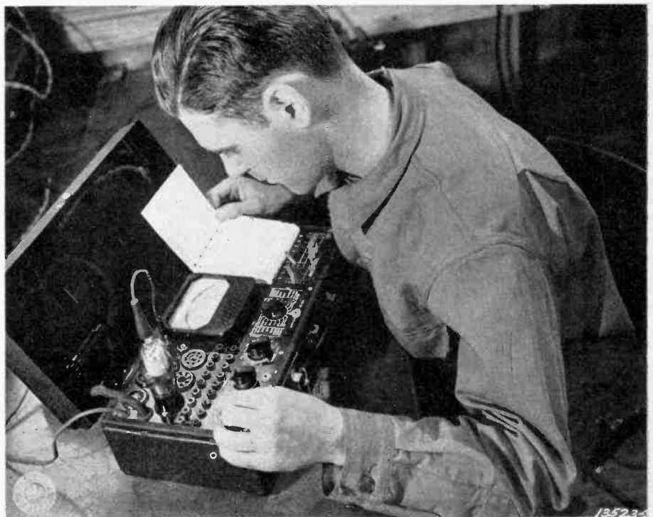
Postwar test sets may be like this one which contains in a single cabinet a tube tester, AC-DC volt-mil-meter & ohmmeter
