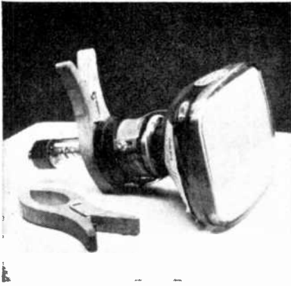
Large wooden clothespins, such as used by electricians and linemen may be modified to support both the yoke and test CRT.
