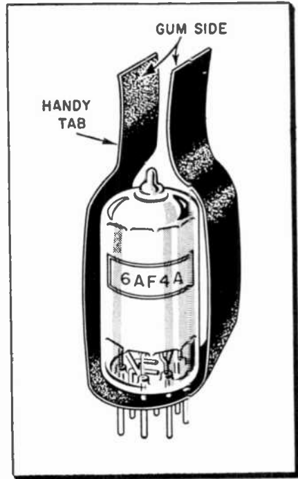
Heat and shield conditions permitting, plastic tape forms handle for miniature tubes.
