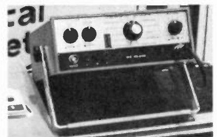
Fig. 10. VIZ's Model WR-515B has video and RF outputs; adjustable video, chroma, and RF output levels and a variety of patterns available.
