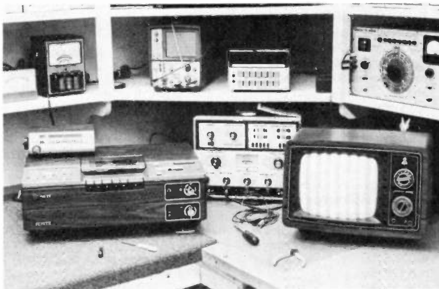
Fig. 7. Sencore's VA48 in action on the author's VCR bench. The VA48 can supply just about any signal needed in any sort of video servicing.
