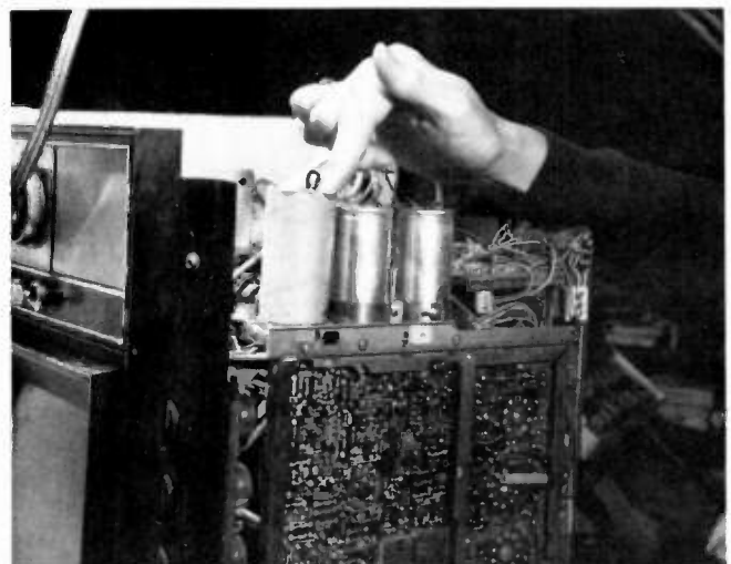
Fig. 5—Don't overlook a dried-up or leaky filter capacitor. These capacitors range from 220 to 1500 mfd.
