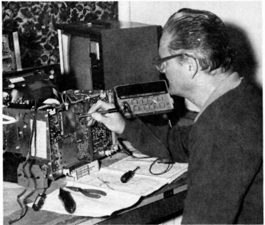
Fig. 1—Here a TV technician is servicing the voltage regulator circuit of a portable color TV.
