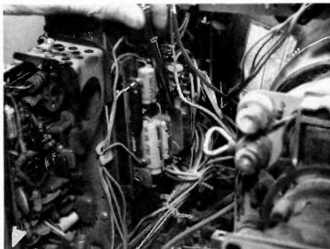
Fig. 4—You may find the voltage regulator circuitry packed or tacked in any place in a Japanese TV receiver. Some of them may be a little difficult to get at for servicing.
