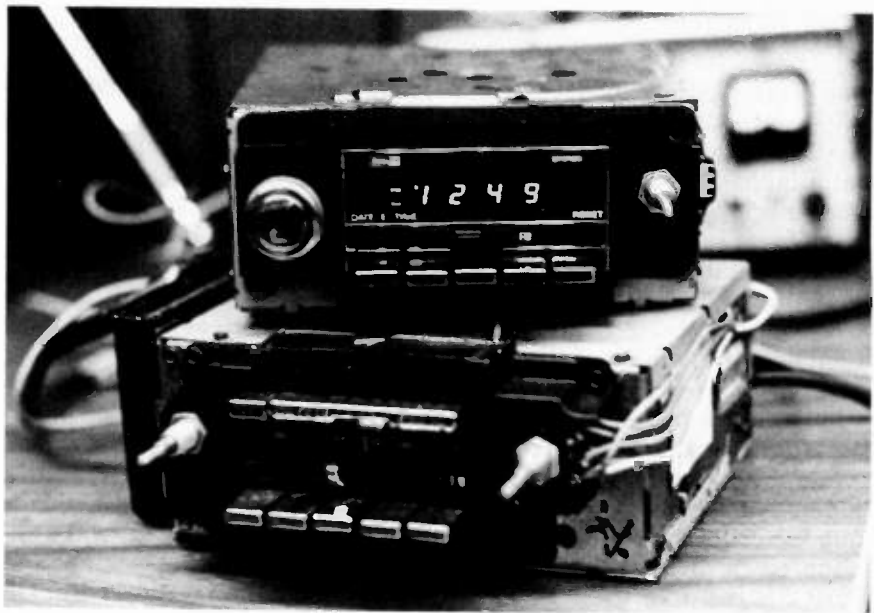
Fig. 4—Delco's digital AM/FM-stereo car radio uses digital circuitry in several areas. It features a digital frequency dial (showing 1249-KHz here), digital clock, digital time, etc. on the same display. This radio is a good example of how digital electronic circuitry has invaded the consumer field in areas that were once the exclusive preserve of analog.
