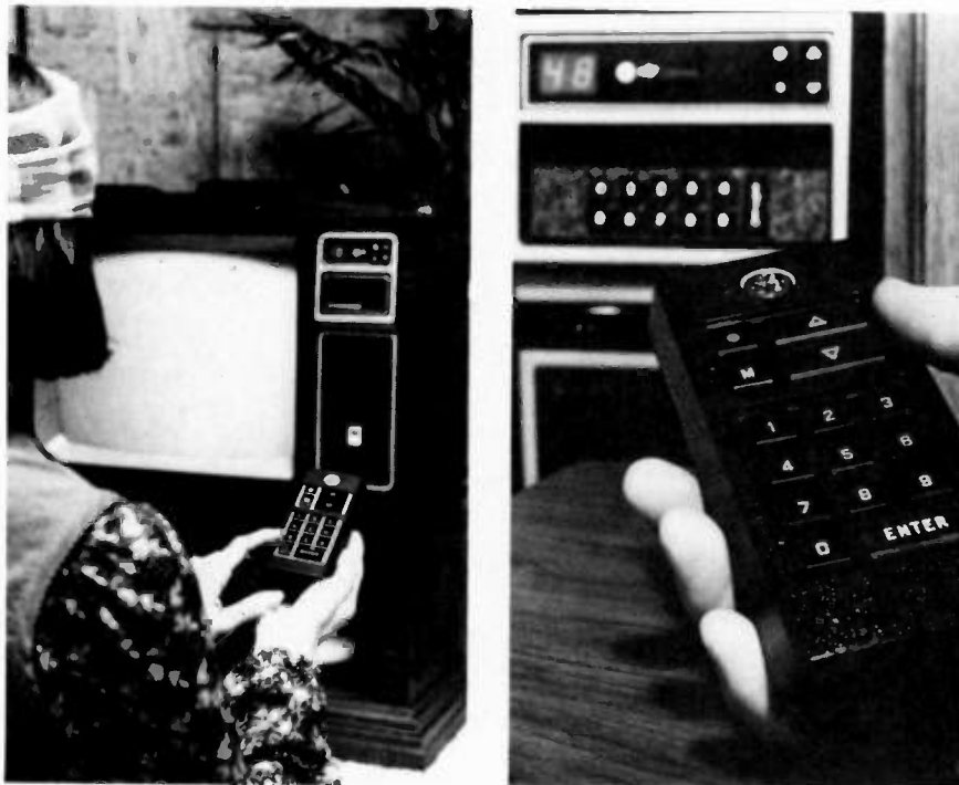
Fig. 1—GE's new remote control unit that uses infrared light to control their new electronic tuning system. Remote unit is on the left. Controls are repeated on the front panel of the receiver (right).
