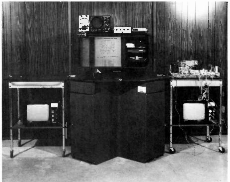
Fig. 5—This is the new GTE Sylvania Electronic Work Station, a free-standing, self-contained unit requiring only electrical and antenna connections.
