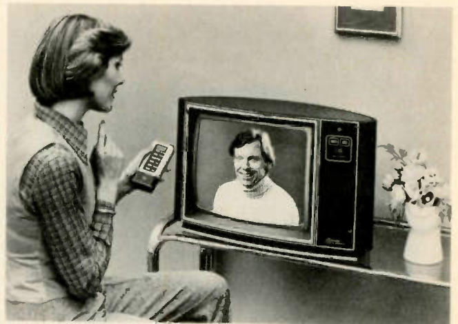
Fig. 8—Elliptical styling highlights this 19 inch "slim line" table model from Zenith for 1978. Remote control, in-line, 100 degree CRT, and Space Command with "Zoom" feature are included in this Model SJ1951W.
