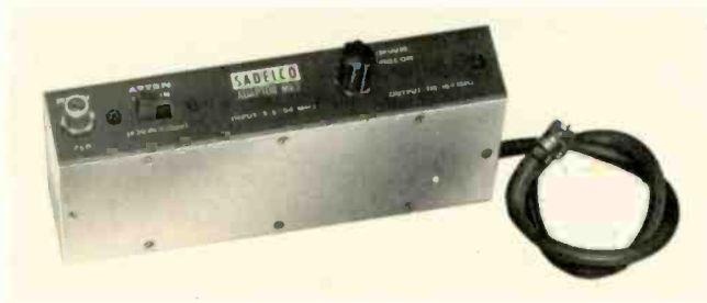
Fig. 15—A typical low-frequency adaptor, MK-2, that converts incoming 4.5 to 54 MHz frequencies to 115 to 164 MHz, which are then read on the SLM's midband scale. Battery powered, the unit slips into the accessory compartment of the FS-780B SLM.
