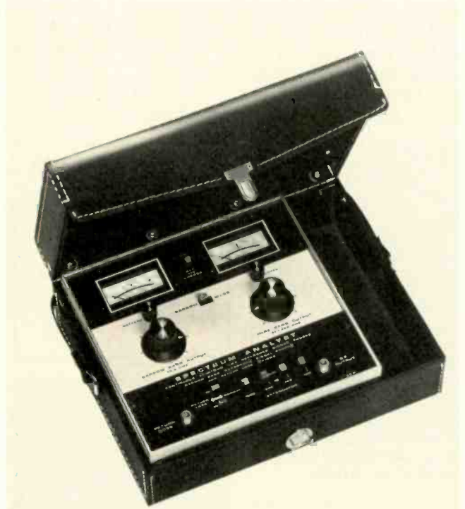
Fig. 16—This Spectrum Analyser, Model 260A, emits a continuous, flat signal from 4.5 to 300 MHz, uniform to within \pm 1 dB throughout its frequency range. A built-in 75-ohm comparison bridge permits direct measurements of return loss.
