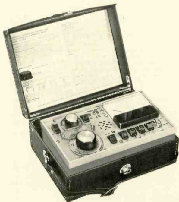
Fig. 1—A typical signal-level/field-strength meter, Winograd Model FS-780B, that provides measurements of all VHF ( \pm 1 dB), UHF and FM carriers in the 10-microvolt to 2-volt range.
