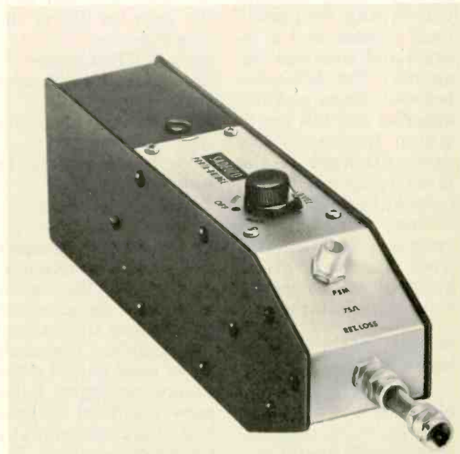
Fig. 18—This is a Porta-Bridge, Model PB-1, a portable 75-ohm comparison bridge that also generates a continuously flat signal ( \pm 1.5\text{dB} ) to permit direct measurements of return-loss and VSWR.
