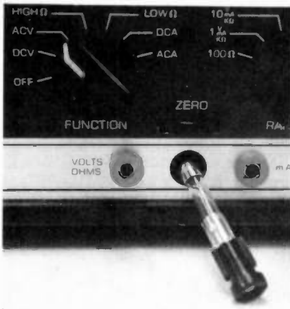
Close-up view of right-hand side of the 283's front panel showing input protection fuse removed. (Fuse is installed in 'common' input jack. Twisting spring-loaded jack with tip of finger releases it, causing fuse to pop out.)
