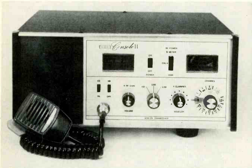
Fig. 1—Example of a Citizen Band SSB base-station transceiver. Mode switch allows selection of AM, upper or lower sideband. "Clarifier" adjusts the locally generated carrier in the receiver for best recovered audio. BFO frequency is critical to within a few Hertz. (Courtesy of SBE.)
