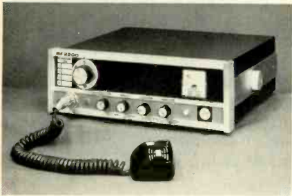
Fig. 10—Examples of a high-frequency SSB transceiver. (Courtesy of RF Communications.)
