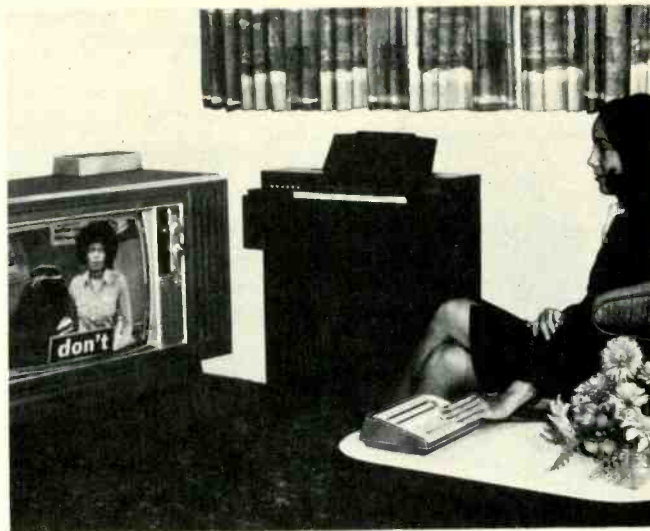
Jerrold's TRC-12 universal TV remote control system. Unit on Top of the receiver is the RF converter, and the unit on the chair-side table is the control unit.
