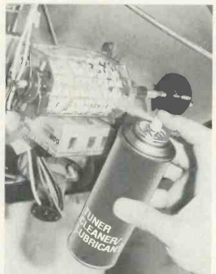
Fig. 2—The second step in proper tuner cleaning and lubrication: Spray all contacts with a cleaner/lubricant and then rotate the rotor a few times while checking to see that the stator contacts press against the rotor contacts with sufficient pressure to insure a positive contact and a good rubbing (cleaning) action.
