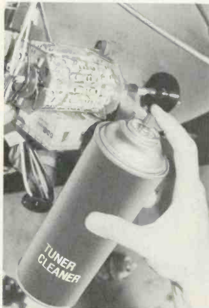
Fig. 1—The first step in proper tuner cleaning and lubrication: Remove the tuner, open it up and carefully spray all of the contacts with a tuner cleaner. Then wipe with a clean, lint-free cloth.
