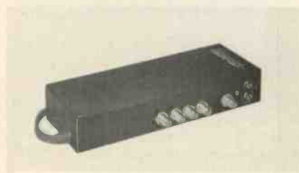
BC-274 Booster Coupler divides the input signal four ways and provides 6 dB gain to each of the 75-ohm outputs. Its high-level input (0.2 volt) allows it to operate as an amplified 4-way splitter following a distribution amplifier. It is designed to supply signals to four TV sets, usually via wall outlets.
