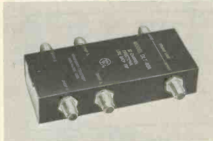
DLT-10A, -20A and -40A Directional Line Drop Tap attenuates reflected signals to tap outlet, entering from trunkline output, by 27 dB average. Each drop supplies a single wall outlet or a feeder line to several wall tapoffs.
