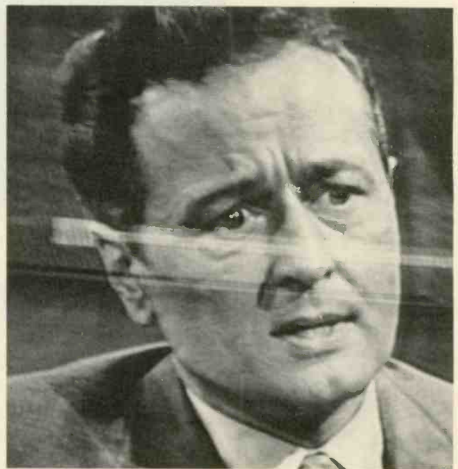
Fig. 5—Cross-modulation interference, shown here, is caused by a strong local TV signal during reception of a distant signal on the same channel.
