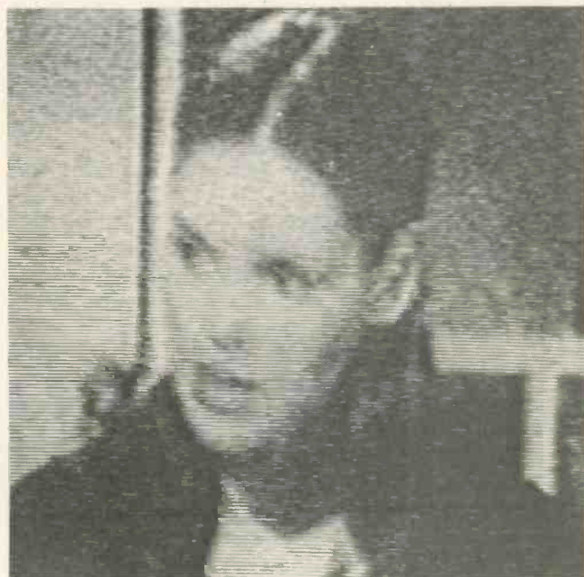
Fig. 9—"Snow" is actually noise which appears on the TV screen as tiny white dots, and is caused by a weak signal.
