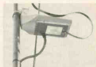
Fig. 10—Solid-state mast-mounted preamplifier.
