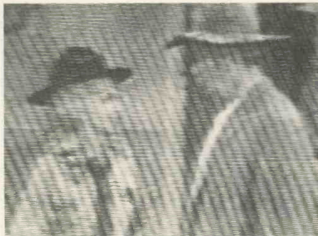
Fig. 7—The interference shown is caused by Ham, CB, or Police band radio transmissions.
