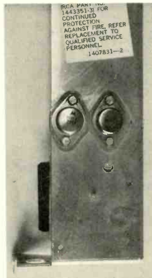
The vertical-output transistors are mounted on a large heat sink, fastened to the main chassis.
