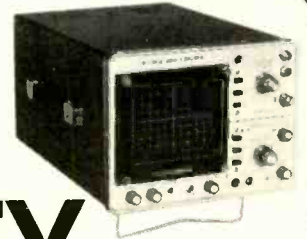
LBO-502 — 5" Solid State Triggered Scope
