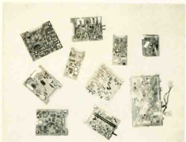
Approximately 66 percent of the set's total electrical components are found on these 10 plug-in modules.
