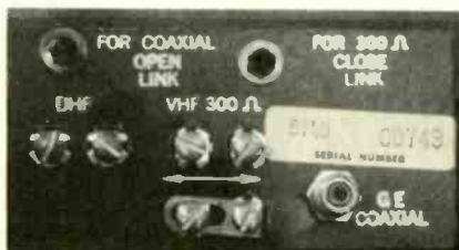
Provisions are made to accept a 75Ω coaxial cable antenna system. A 300Ω VHF input is provided via a 75Ω-to-300Ω balun, which is connected by means of a shorting link.
