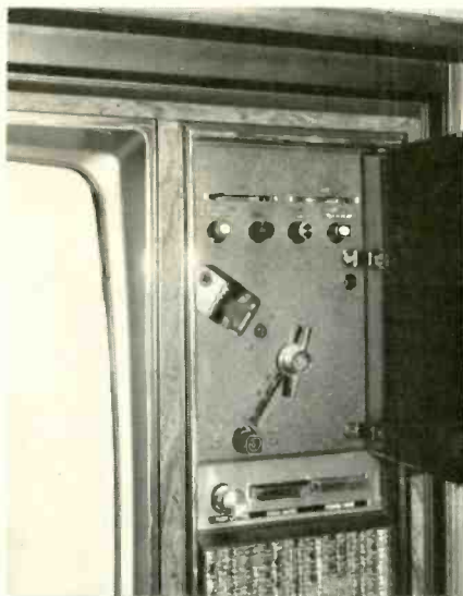
Only the essential customer controls appear on the front panel, the less important secondary controls being hid behind the panel door.
