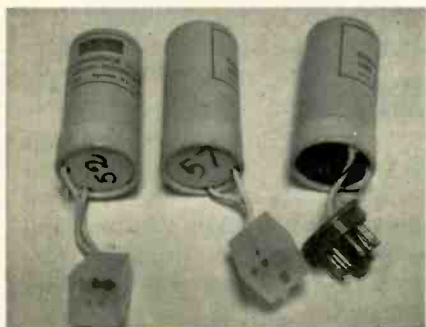
TeleMatic's convergence loads have sockets to match most color-TV chassis. The one at the right is supplied with the test jig.
