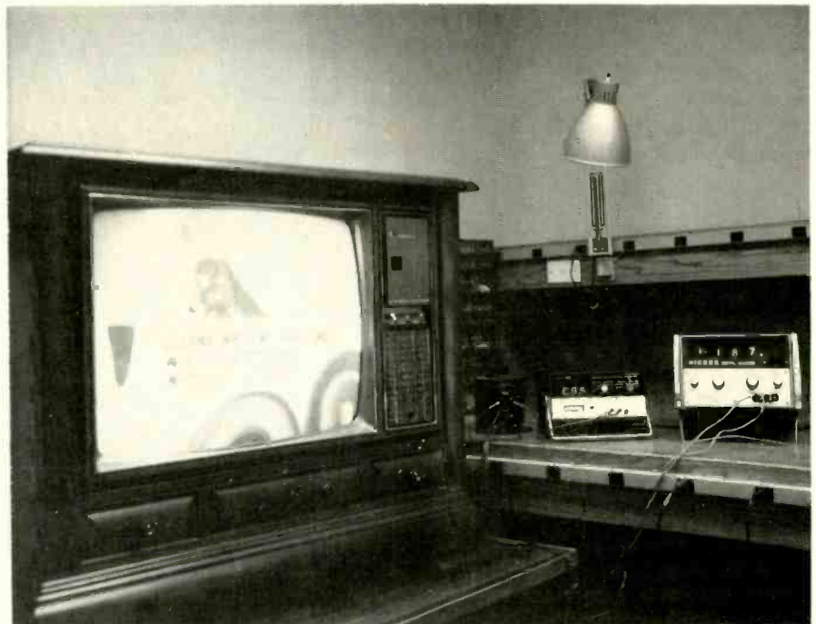
Fig. 4—The TV set ac line voltage was reduced to 85v and still we obtained a full-screen color raster.
