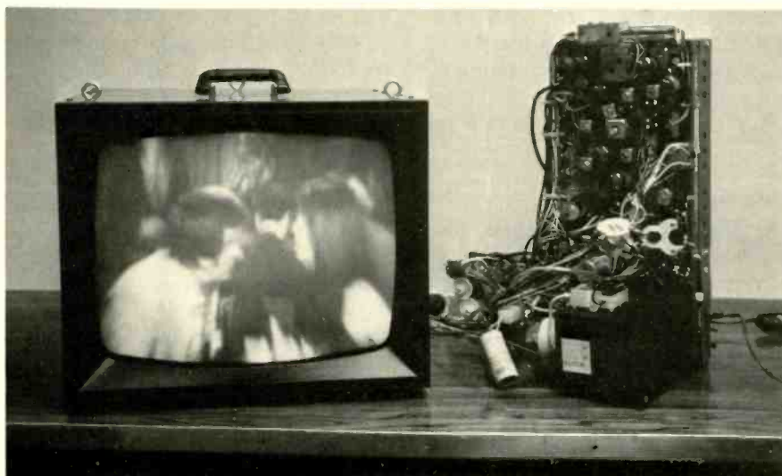
Actual well proportion picture obtained on the color-TV test jig when connected to the Admiral 1K18-1A color-TV chassis.
