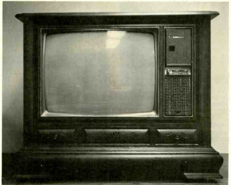
Motorola's Model TU945HS Color-TV set employing the ATS-938-A06 chassis with a simplified, one-panel remote-control system.
