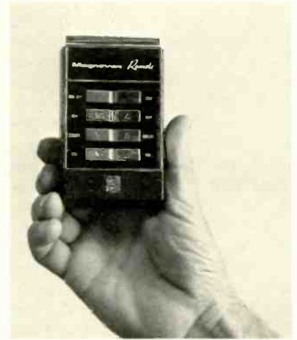
The remote control transmitter is compact and controls eight TV functions.
