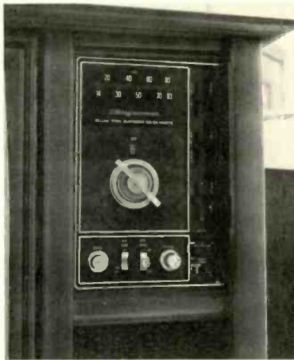
A control panel door hides most of the controls on the front panel.
