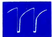
21 200 VOLTS P/P, 15,750 HZ PIN 6 V42
