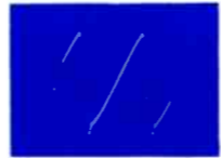
17 16 VOLTS P/P, 15,750 HZ D41 TOP END
