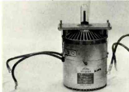
M4545A Magnetron Tube (note cooling fins). Courtesy of Sharp Electronics Corp.
