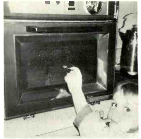
Illustration of how a child can easily push a safety pin through oven grille while the oven is in operation, exposing herself to serious danger.
