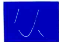
14 10 VOLTS P/P, 60 HZ PIN 9 V41
