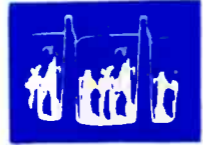
9 6.6 VOLTS P/P, 15,750 HZ BASE OF Q41
