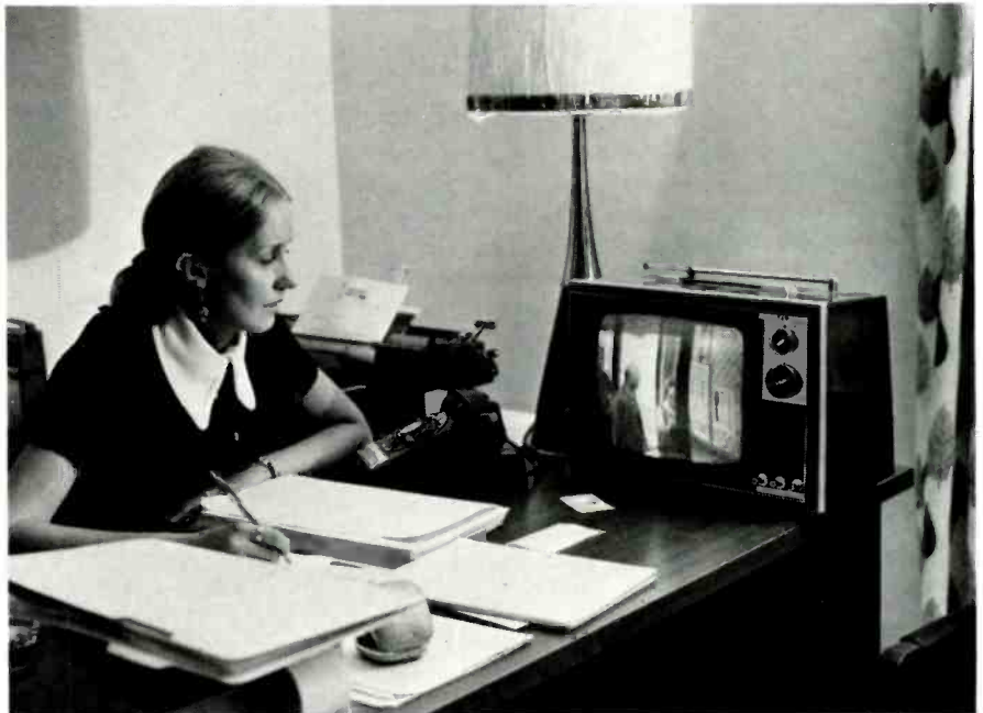
Fig. 6—Secretary in rental office monitors arrival of visitor in lobby of Lansdowne Towers, a luxury apartment complex in Upper Darby, Pa. This CCTV system, tied into the MATV system in each building in the complex, permits residents to identify callers before admitting them to the building.
