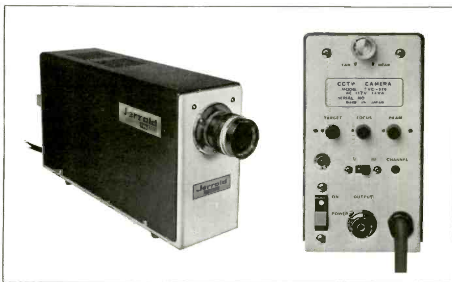
Fig. 4—A compact TV camera, such as the Jerrord Model TVC-500, is ideal for home CCTV systems, since it develops clear, sharp, B/W pictures and delivers them in either video or RF signal format. When switched to video format, the camera delivers its signal to a video monitor; while when switched to RF format, it feeds the signal to a standard TV set. A screwdriver adjustment permits the user to select the desired frequency for display on Channels 2 through 6.
