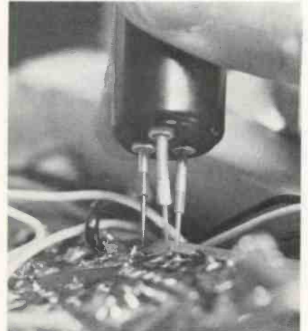
Fig. 2—The blue tip is pressed down first against the collector connection. Pushing lightly on the probe barrel causes the point to penetrate to the solder.
