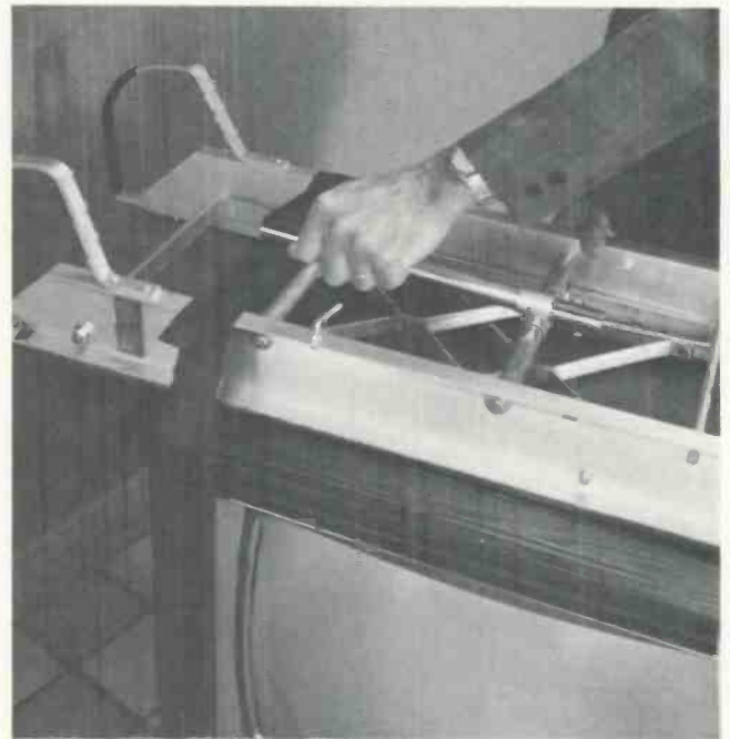
Fig. 9—Swinging a clamp at the top of the hand truck tightens a security belt around the console TV set and truck.
