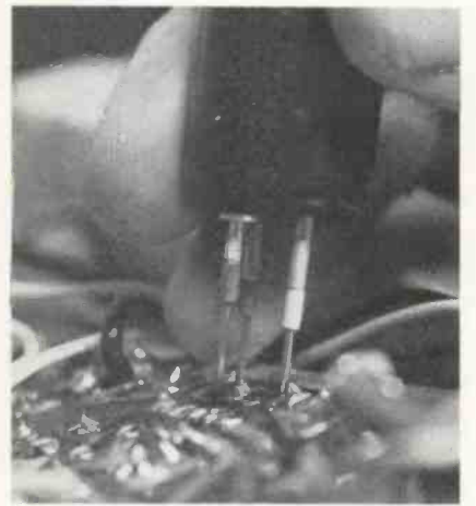
Fig. 3—The yellow tip is applied to the emitter connection next. A spring-and-ball socket keeps the blue tip in place while positioning the yellow tip.
