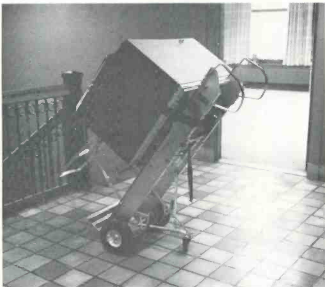
Fig. 3—The third wheel is capable of making the loaded hand truck self-supporting.
