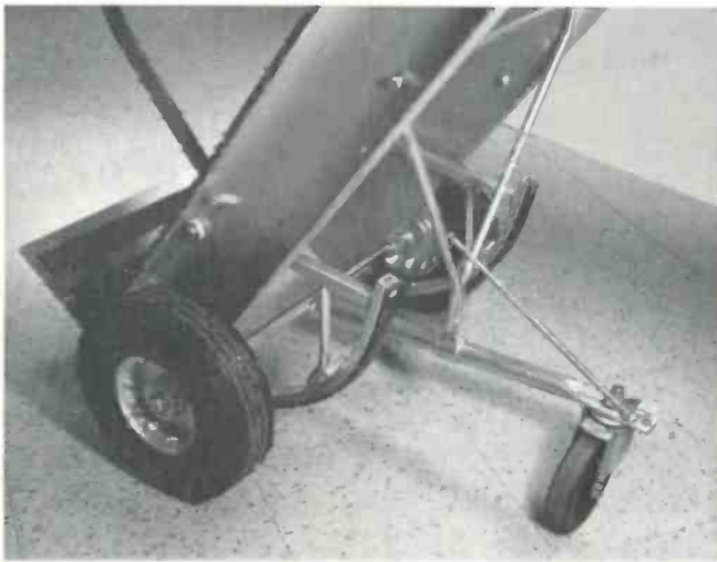
Fig. 2—Third wheel and swivel breaking system are extra features included on the hand truck.
