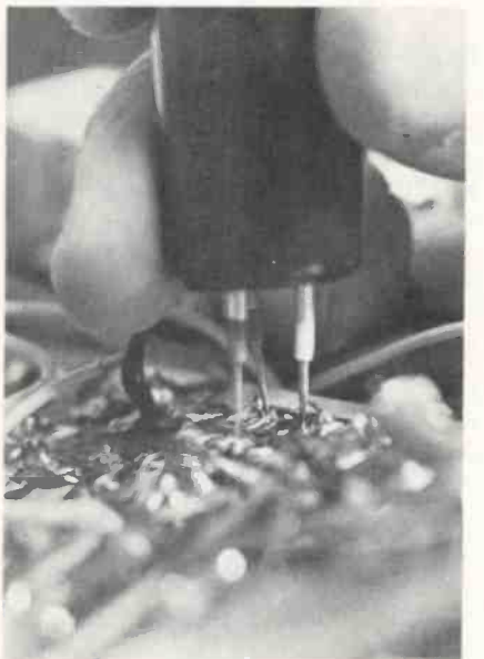
Fig. 4—The green tip makes the base connection after the collector and emitter have already been positioned.
