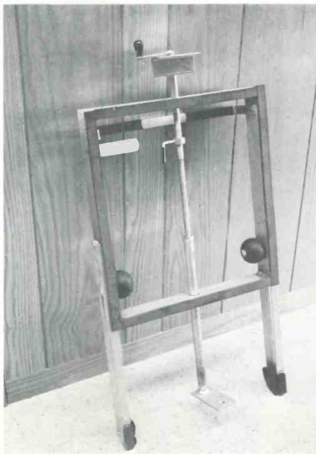
Fig. 5—The tilting cradle increases the versatility of the hand truck.
