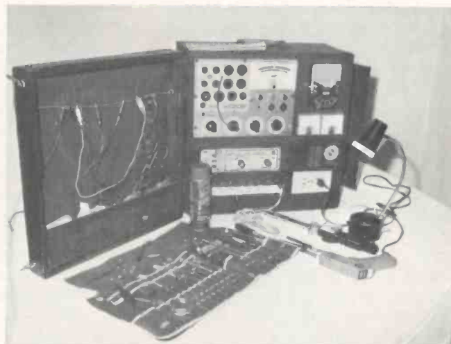
Fig. 2—Once opened in the home, this service lab simplifies the task of preparing to work on a defective electronic consumer product.
