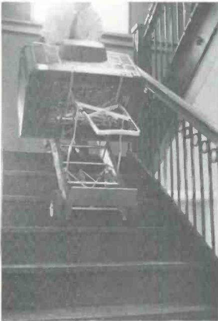
Fig. 3—The third wheel is capable of making the loaded hand truck self-supporting.
