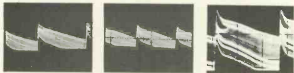
Fig. 45—Signal present at the transistor base in the pincushion-correction circuit. The waveform on the sync-sweep scope (left) was not as easily seen as that shown by the trigger-sweep scope (center).
