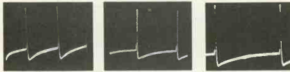
Fig. 33—Differentiated signal near the vertical hold control, as indicated by the manufacturer (right), and as seen on the trigger-sweep (center) and sync-sweep (left) scopes.
