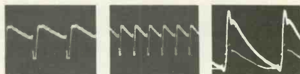
Fig. 18—Signal obtained from sync amplifier circuit, as indicated by manufacturer (right), and as seen on the trigger-sweep (center) and sync-sweep (left) scopes.
