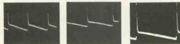
Fig. 37—Signal at the plate of the vertical output tube, as indicated by the manufacturer (right), and as shown on the trigger-sweep (center) and sync-sweep (left) scopes.
