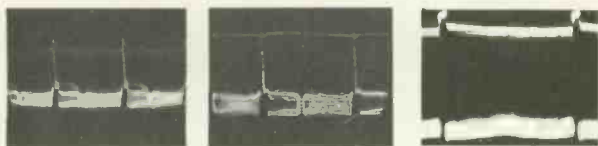
Fig. 12—Amplified signal remaining after sound has been removed, as indicated by the manufacturer (right), and seen on the trigger-sweep (center) and sync-sweep (left) scopes.
