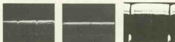
Fig. 15—The amplified sync signal used for synchronizing the vertical and horizontal oscillator circuits, as indicated by the manufacturer (right), and seen on the trigger-sweep (center) and sync-sweep (left) scopes.
