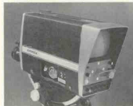
Fig. 12—The Ampex CC-326 series studio camera features a 9-in. viewfinder and a 25mm, F9.5 lens. The camera frame and operating features are identical in all models of this series.
