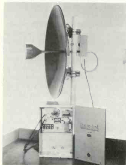
Fig. 4—2500MHz transmission (above) and receiving (below) equipment for an instructional television network.
