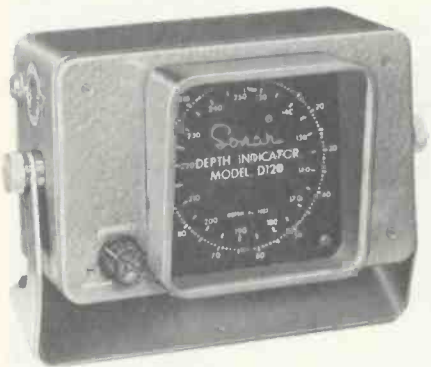
The Sonar Model D120 Depth Indicator is tube operated for use on 6 or 12vdc and provides readings to 250ft on two scales. (Courtesy Sonar Radio Corp.)
