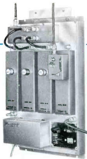
UHF converter may be plugged directly into single channel headend strip. Courtesy Winegard.
