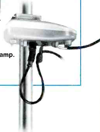
UHF converter may be plugged directly into single channel headend strip. Courtesy Winegard.
