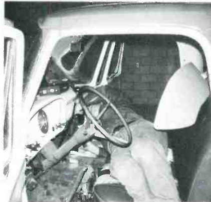
Installation technician mounts transceiver bracket to dash panel.
