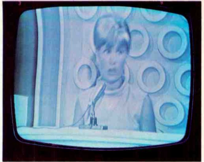
Fig. 4—Color picture with only a green tint showing. Notice the extremely green fringing at the left side. Nine times out of ten, this condition is caused by the 3.58MHz reference oscillator failing.
