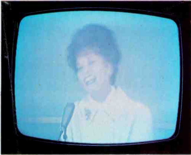
Fig. 3—A typical screen of a color set indicating loss or weak color. Even with the color killer wide open, all color tubes substituted, color signals were still weak.
