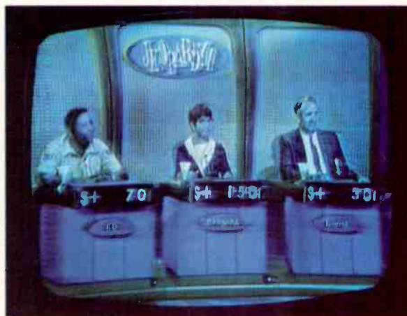
Fig. 7— Red was missing from this color picture because of a leaking coupling capacitor from the "X" demodulator plate to the R-Y amplifier grid.
