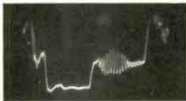
One horizontal sync pulse with its color burst.
