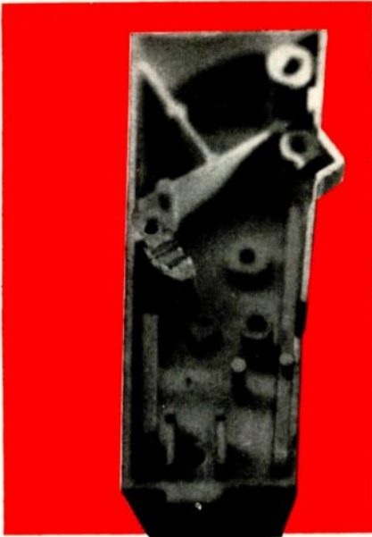
The plastic at the pivot point can be broken if too much upward pressure is applied.
