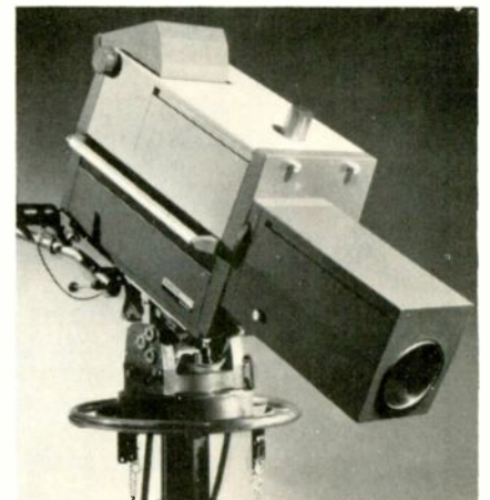
This fully transistorized color television camera manufactured by Marconi uses four plumbicon pickup tubes. The camera can be switched to either the 525 line or 625 line standards and will provide signals suitable for coding to any of the systems that have been proposed—NTSC, PAL or SECAM.
