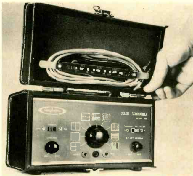
Amphenol's compact, solid-state color generator fits into tube caddy.
