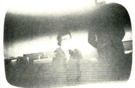
Fig. 4 (B)—A 120 cps ac signal causes two bars in picture — usually because of filter leakage in full-wave power supply circuits.
