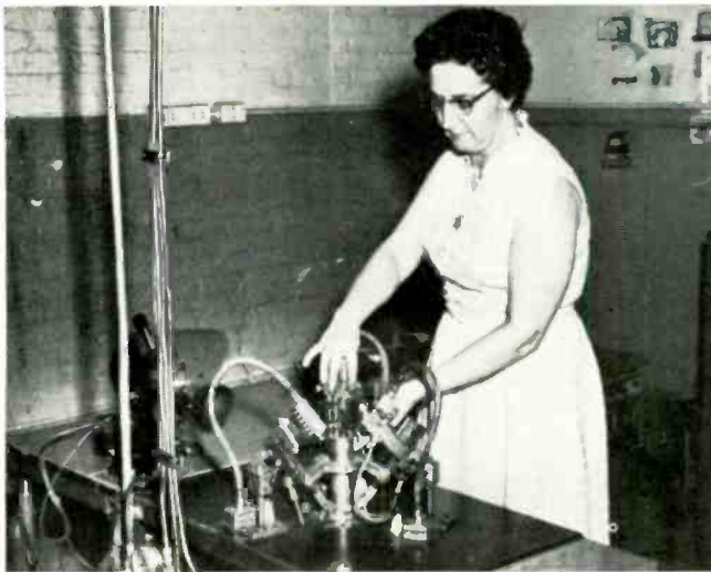
Beading machine is used to produce electron guns — three for each CRT....
