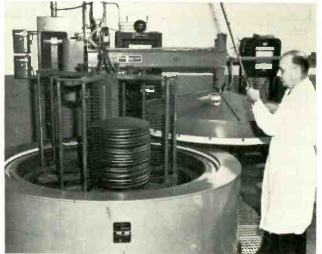
Aperture masks are lowered in a steam tank for blackening. Process increases thermal radiation properties....
